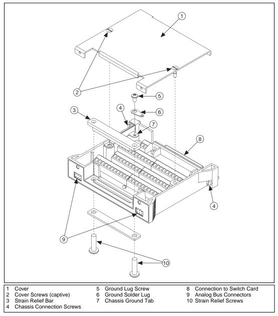
Figure 1. TB-2606 Parts Locator Diagram
