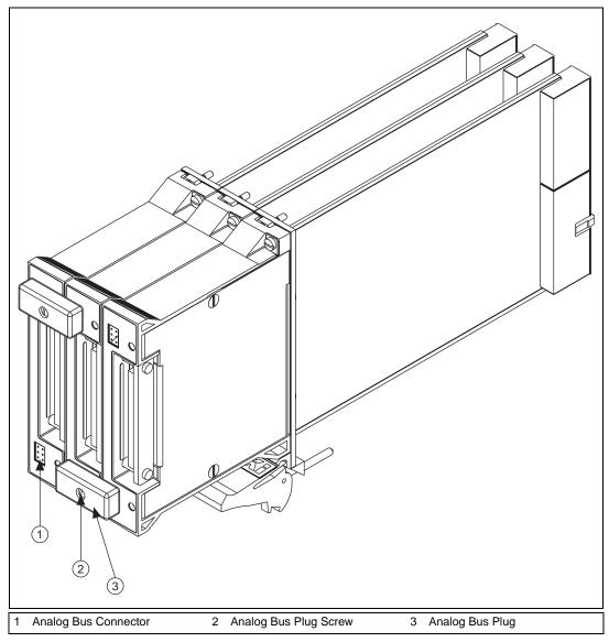
Figure 3. Installing the Analog Bus Plug
