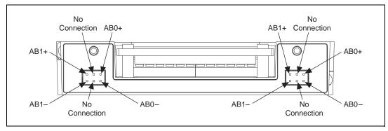
Figure 4. Analog Bus Connector
