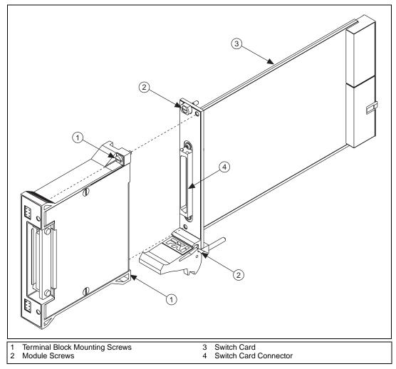
Figure 2. Connecting the TB-2606 to the Switch Card
